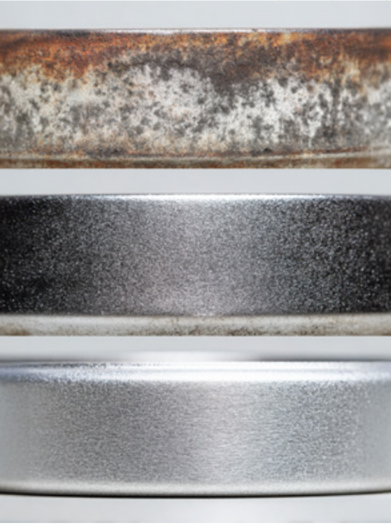
Top to bottom: Workpiece prior to surface treatment, workpiece after using glass blasting granulate, surface finish using glass blasting beads. Photo credit: Studio 0816, Midjourney
