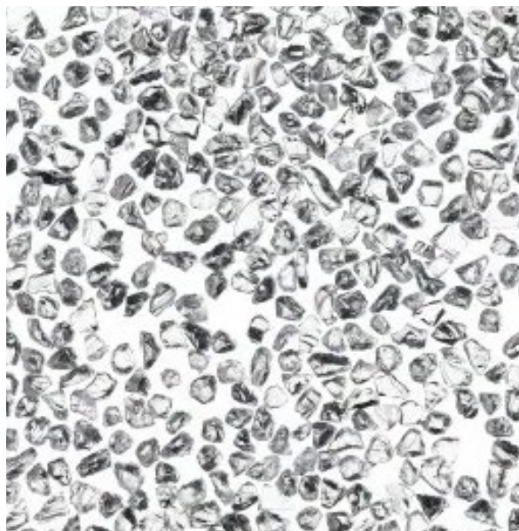
The granulate's sharp-edged structure allows for quick and thorough cleaning of metal surfaces. Photo credit: SWARCO Indusferica
