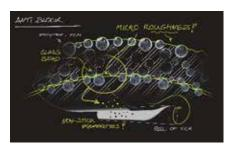
With glass filler beads, it is possible to obtain a certain micro-roughness of the film surface, and thus, prevent blocking in rolls.
