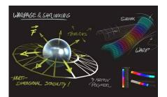
Glass beads improve warping and shrinking properties of thermoplastics.
