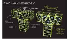
In plastics processing, the use of glass beads reduce sink marks.
