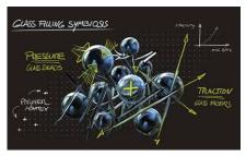
Hybrid combinations of glass beads and glass fibres combine the advantages of both reinforcement materials.
